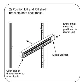
4) It is essential that the centre of the runners on the bracket and rollout fitting are correctly aligned before pushing in rollout fitting
