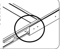
5) Once runners are aligned gently push the centre of the rollout fitting towards unit. Once the fitting has clicked into place, move the fitting backwards and forwards to check it is correctly fitted before using
