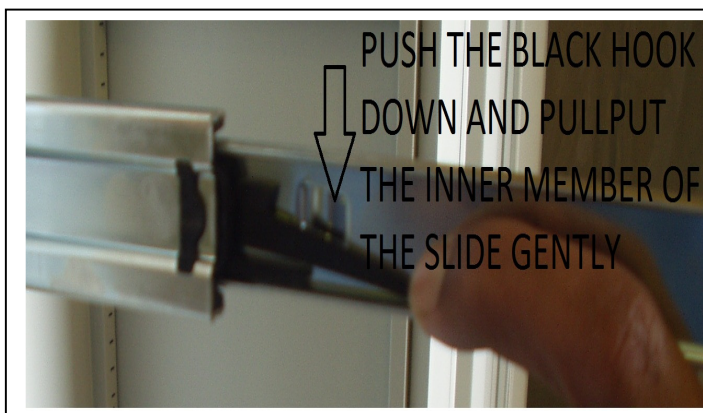
STEP 5: PULLOUT THE INNER SLIDE MEMBER OF THE LH SLIDE BY PRESSING THE BLACK HOOK DOWNWARDS AS SHOWN
