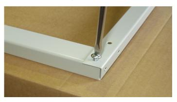
STEP 4: ASSEMBLE THE OTHER SHORT MEMBER WITH THE OTHER END OF THE SAME LONG MEMBER USING SCREW
