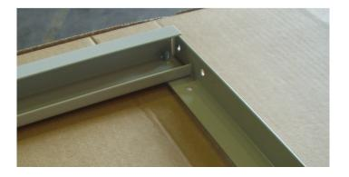
STEP 6: ENSURE THE POSITION OF THE SCREW AS SHOWN IN THE ABOVE PICTURE (FIX END OF SHORT MEMBER)
